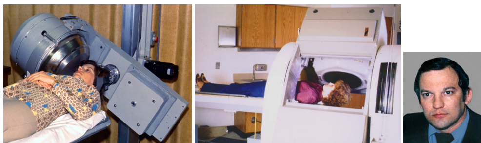
Figure 6. Ron Jaszczak and the Searle rotating-camera SPECT scanners: (left) brain imager; (middle) dual-camera, whole-body SPECT system.
